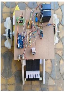
multiple components, including sensors like the ultrasonic sensor and ESP32 camera, motors, motor driver like the L293d, LM2596 and the Arduino UNO-based controller, enables the
